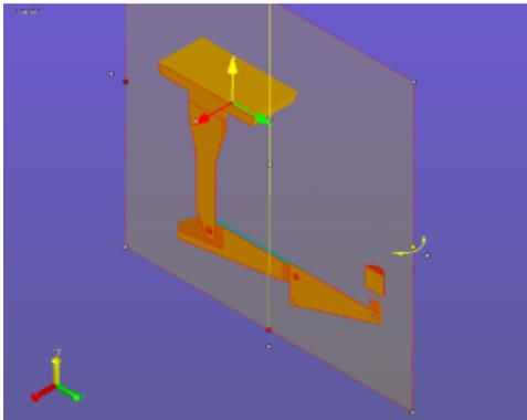
To slide the plane along the normal axis, click and drag one of the white grippers located in the center of the plane and at each corner. Yellow direction arrows appear indicating in which direction you can move the plane.
