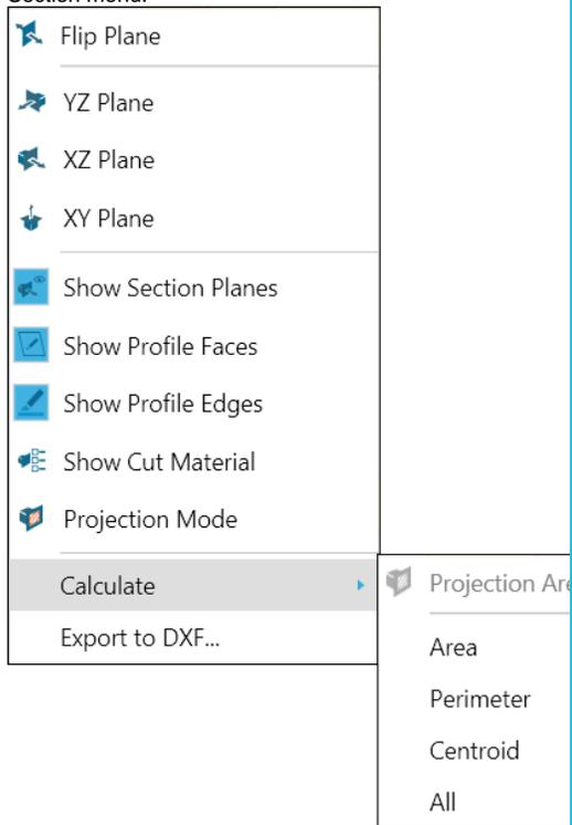
2. Mouse over the **Calculate** selection, and make a selection from the flyout menu. (Projection Area is active only if Projection Mode is enabled.)
