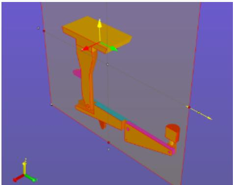
To *rotate* the plane around a horizontal or vertical axis, click and drag one of the red grippers located in the center of each edge. Yellow direction arrows appear indicating in which direction you can move the plane.
