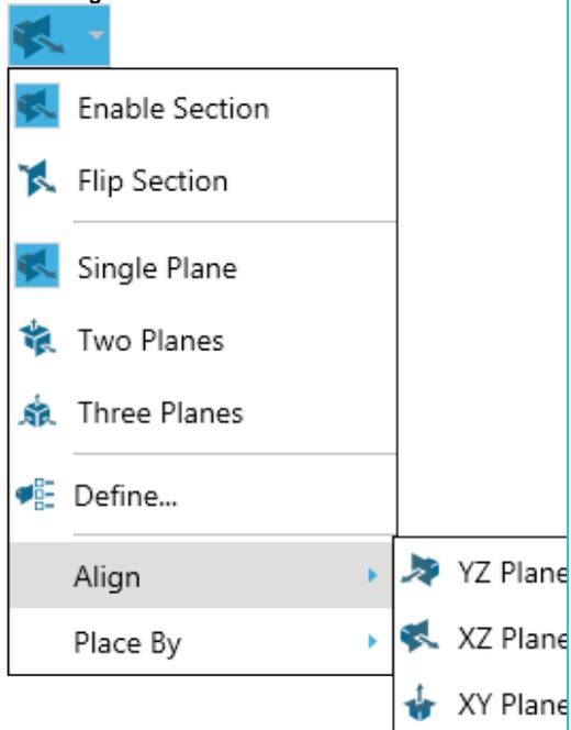
3. Click either **XY Plane**, **XZ Plane**, or **YZ Plane**. The red dots on the model designate available vertices on the model. A cross-hatch appears when the pointer is properly positioned over a vertex point.
