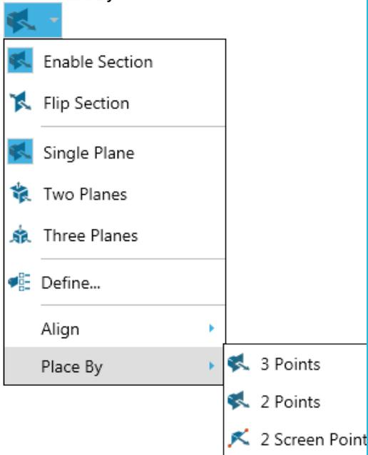
3. Click **3 Points**. The red dots on the model designate available points on the model. A cross-hatch appears when the pointer is properly positioned over a point.
