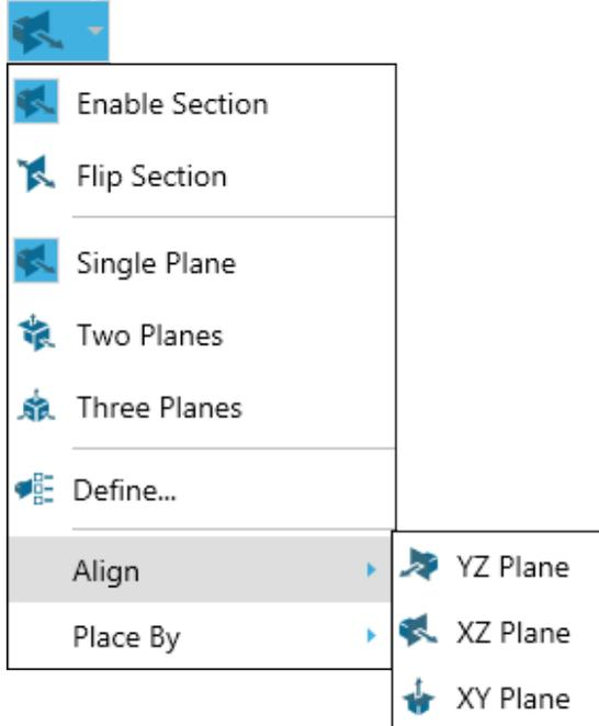
3. Click either **XY Plane**, **XZ Plane**, or **YZ Plane**. The red dots on the model designate available vertices on the model. A cross-hatch appears when the pointer is properly positioned over a vertex point.
