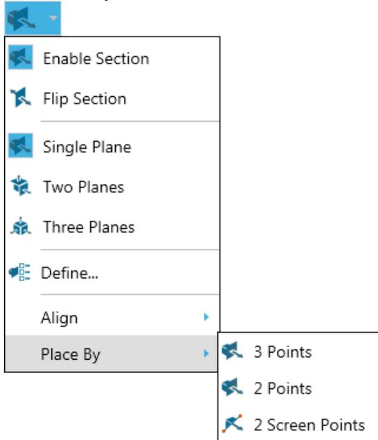
3. Click **3 Points**. The red dots on the model designate available points on the model. A cross-hatch appears when the pointer is properly positioned over a point.
